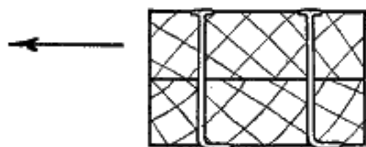
FIG. 73.—Clinched nails. If forces tend to move the top board to the left, then the points of the nails should be bent over to the right.
