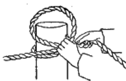
FIG. 340.—The timber hitch and half hitch combined.
