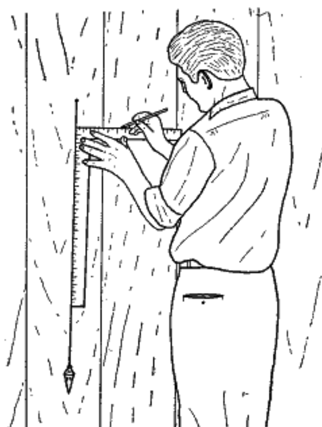
FIG. 18.—Establishing a level line by means of a plumb bob and square.
