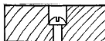
FIG. 84.—Counter-bored holes may be used to sink round-headed screws below the surface.
