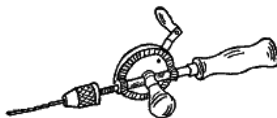
FIG. 192.—The hand drill is one of the most useful tools for drilling small holes, either in metal or wood.
