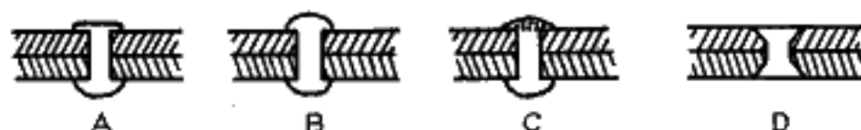
FIG. 188.—Methods of heading rivets.
