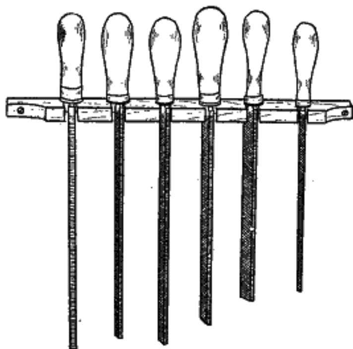
FIG. 171.—A good way to keep files is to hang them by their handles on a rack. A file should not be thrown in a drawer nor on a shelf where the sharp cutting edges might be dulled by contact with other files or tools.
