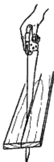
FIG. 27.—If the saw leaves the line, twist the handle slightly and gradually draw it back to the line.
