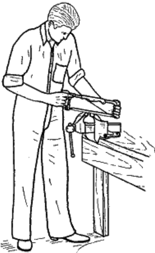
FIG. 179.—In sawing with a hack saw, stand at ease with the right foot 10 or 12 in. back of the left, and with the right forearm, elbow, and shoulder in line with the saw. Use long, even strokes, swaying the body back and forth slightly in rhythm with the arm strokes.
