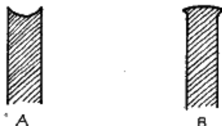
FIG. 131.—A. Shape of scraping burr after burnisher has been used on flat sides of scraper.
