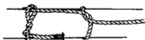
FIG. 340.—The timber hitch and half hitch combined.
