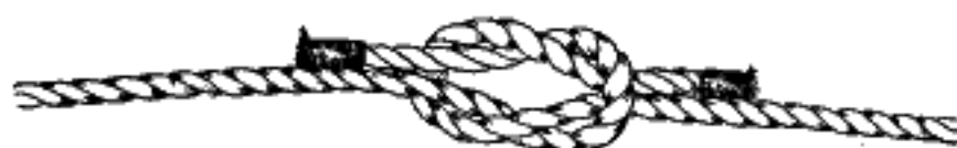
FIG. 326.—The square knot is a very useful knot and should not be confused with the granny knot.
