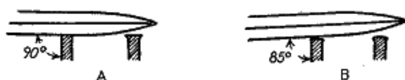
FIG. 130.—In turning the burrs of a scraper, the burnisher is held at 90 deg. to the scraper on the first stroke, and then gradually tilted until it makes an angle of about 85 deg. on the last stroke.
