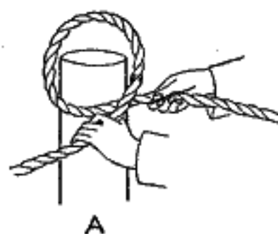
FIG. 339.—The timber hitch.
