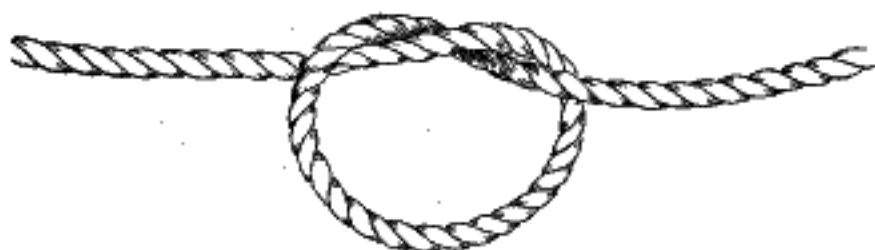
FIG. 324.—The overhand knot.
