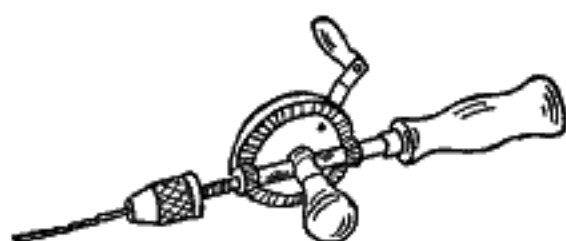
FIG. 65.—The hand drill is a very useful tool for drilling small holes, either in wood or metal.
