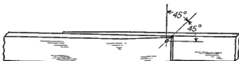
FIG. 303.—The awl makes a diamond-shaped hole. The long axis should be neither lengthwise of the strap nor crosswise, but about halfway between.
