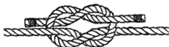
FIG. 327.—The granny knot slips under load and should usually be avoided.
