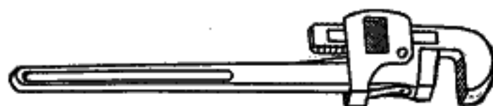
FIG. 211.—Every well-equipped farm shop should have at least one pipe wrench, preferably two.
