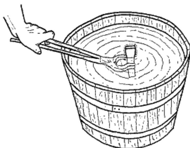
FIG. 259.—When it is desired to heat only a small portion of an iron, as in upsetting only the end of a piece, it is sometimes necessary to heat a larger portion, and then cool back to the desired point by dipping in water.
